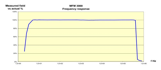
RMS-value presented in measurement display is a wideband value taking onto account all magnetic field components in the frequency range.
