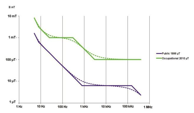
The dotted lines represent the time domain limits and the continuous lines represents the frequency domain limits.
