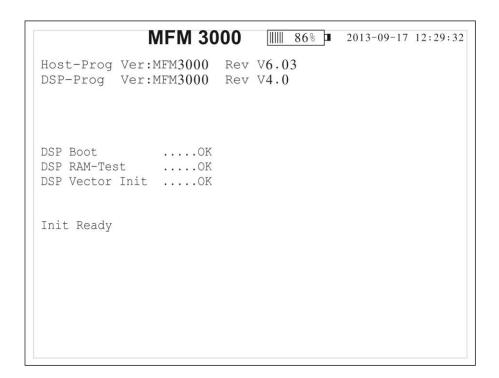
When tests are completed it shows the text "Init Ready" and automatically moves to the measurement display selected last time the instrument was used.
