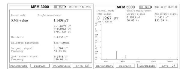
In a sub-menu to "Normal" it is possible (only in **frequency domain**) to reduce the "Bandwidth" if only a limited part of the frequency range is of interest.
