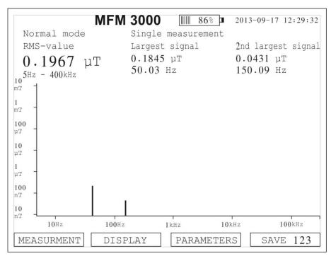
In the spectrum graph in the upper left corner the selection of limits are presented. In this example Normal mode or no limits is selected.
