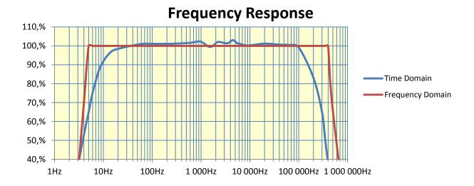
To get the frequency response for the exposure limits from ICNIRP the same technics are used, filtering technic for the time domain measuring mode and detailed individual adjustment of each frequency component for the frequency domain measuring. This will give some different result as it is described in the graph below. Both methods are approaved by ICNIRP.
