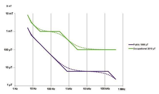
The dotted line is presenting the frequency response when using a first order filter in time domain measurements and the
