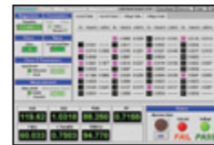
IEC 61000-3-2 Current Harmonic Test (Pre-compliance)
